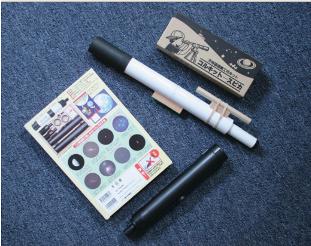
Figure 2 – Two inexpensive telescope kits from Japan offer very good performance thanks to their glass achromatic objectives and compound eyepieces. Either or both of these kits may prove adaptable to the Galileoscope project.
