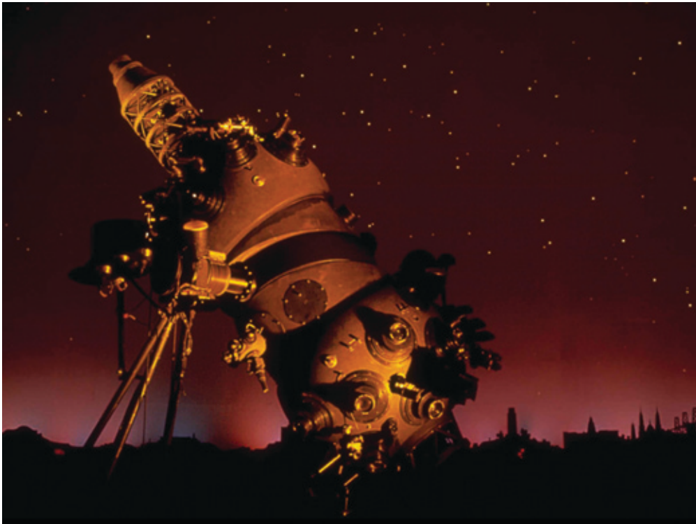
Figure 1 – The original Morrison Planetarium at the California Academy of Sciences in San Francisco, California, USA, featured a unique opto-mechanical star projector. The new Morrison will showcase entirely digital technology.
